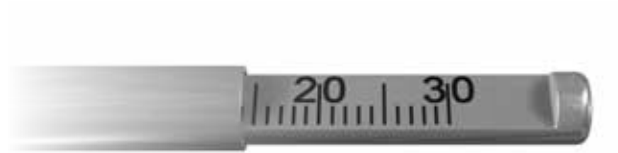
Figure 4 Depth gauge measurement: 14 mm
