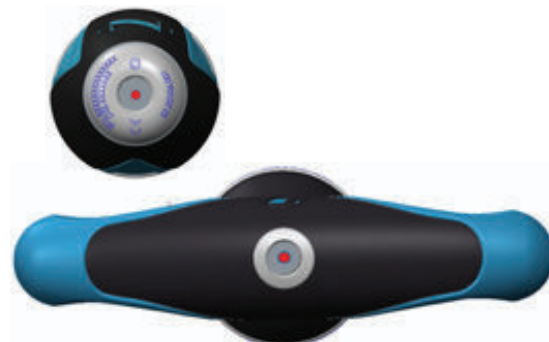
Figure 13: Top down views of standard instrument handles with red spots indicating the approximate location to touch the tip of the passive planar to the instrument during the calibration process.
